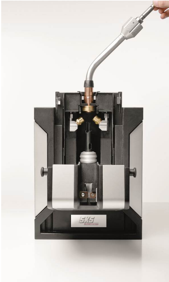
2: eReam, the first 100% electrically driven torch cleaning system (shown with the wire cutter opened) provides fundamental benefits.
