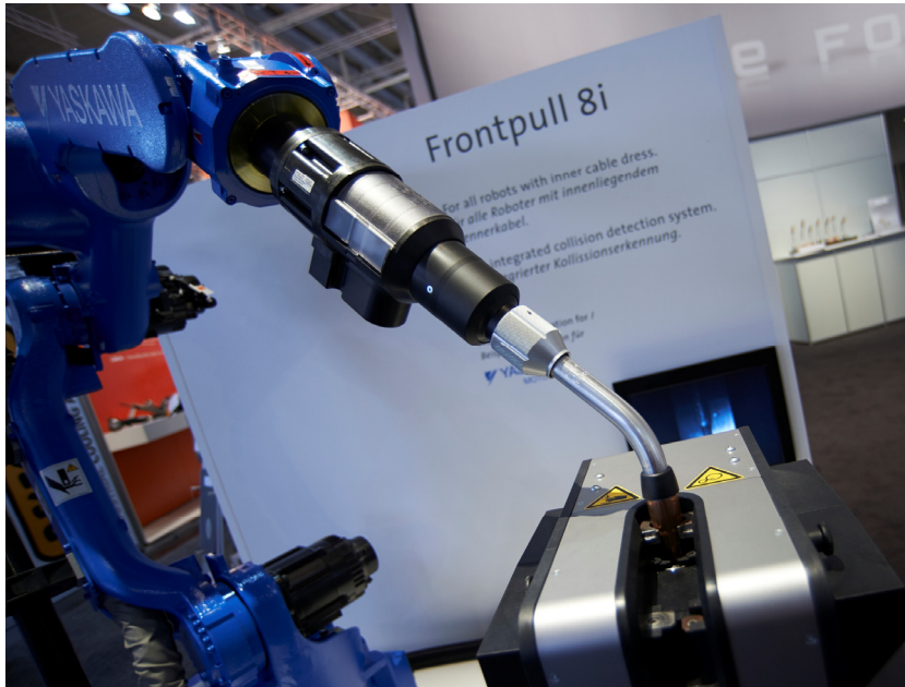
1: Frontpull 8i – the new torch with close-to-process wire feeding and integrated collision detection for process arm robots.
