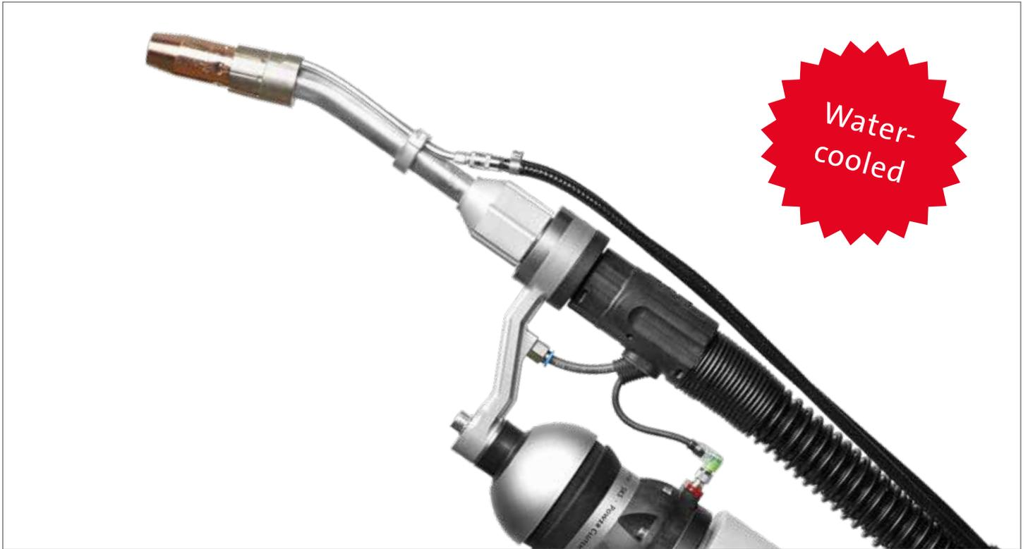
The Power Clutch water-cooled torch system perfects the interaction of welding machines and robots with outer cable dress. The water-cooled Power Clutch torch system consists of the Power Clutch, a mounting flange for each robot type, the torch cable and the water-cooled torch neck with consumables. The changing of the torch neck is designed to be tool-free. This allows for a TCP accuracy of  $\pm 0.2$  mm when changing torch necks.
