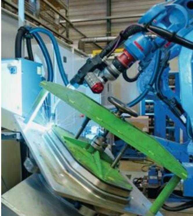
1: The Frontpull 7 feeds even "difficult" welding wires for automated arc welding and soldering with highest precision.
