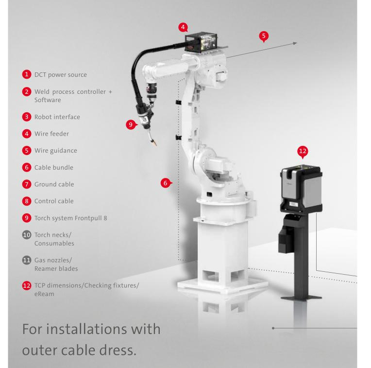
This brochure contains information about the SKS Weld Package, the torch system **Frontpull 8**, as well as consumables and spare parts. There are various features of the welding machine components and torch systems available depending on the robot system and the welding task.
