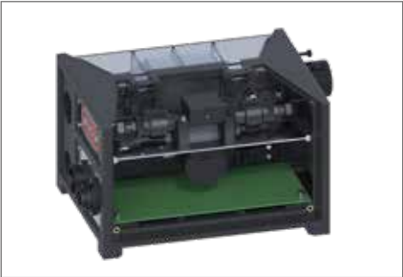
FP8i Module with integrated gas flow sensor
