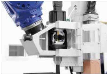
Integration Frontpull 8 into the Laser-Hybrid system
