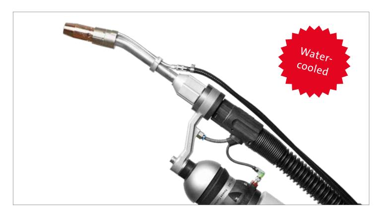
The Power Clutch water-cooled torch system perfects the interaction of welding machines and robots with outer cable dress. The water-cooled Power Clutch torch system consists of the Power Clutch, a mounting flange for each robot type, the torch cable and the water-cooled torch neck with consumables. The changing of the torch neck is designed to be tool-free. This allows for a TCP accuracy of ± 0.2 mm when changing torch necks.
