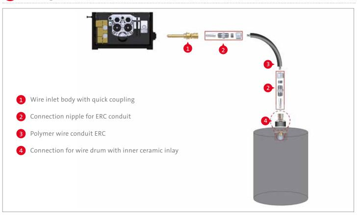
With the ERC wire guidance for steel/stainless steel, the high efficiency of the whole system extends up to the drum.
